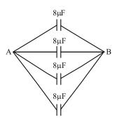
Equivalent capacitance =  $4 \times 8 = 32 \mu F$ .
